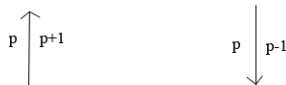
Figure 3.23: The rule for the increase or decrease of indices in an Alexander indexing.
